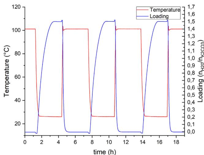
Fig. 4. Cyclic loading of the  $K_2CO_3$  composite at 12 mbar as measured with TGA. The red line indicates the material temperature and the blue line the loading. Full loading of 1.5 mol  $H_2O/mol K_2CO_3$  is reached. (For interpretation of the references to color in this figure legend, the reader is referred to the Web version of this article.)
