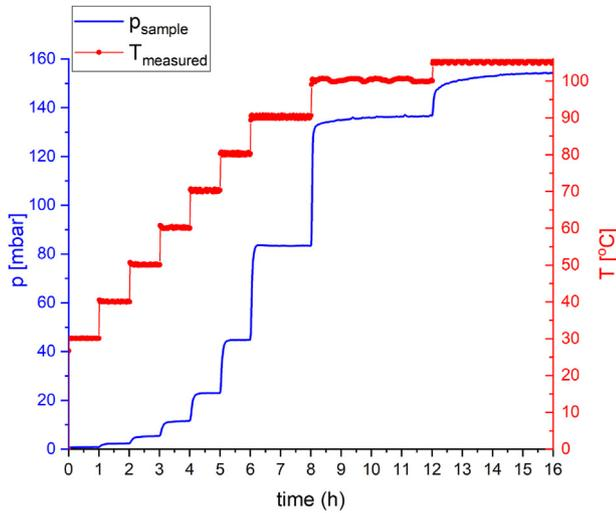
**Fig. 8.** Typical pT measurement with the sample pressure on the left y-axis (blue solid line) and the sample temperature (red dotted line) on the right y-axis as a function of time. The equilibrium line is obtained from the equilibrium pressure at the end of each temperature step. (For interpretation of the references to color in this figure legend, the reader is referred to the Web version of this article.)
