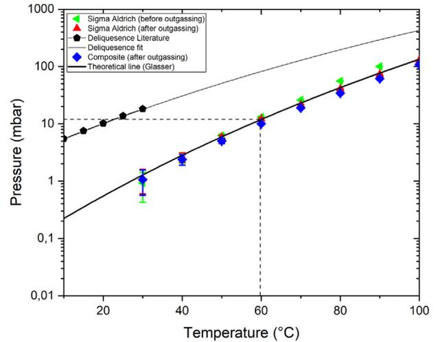
**Fig. 9.** Equilibrium phase transition lines as measured with the pT-setup. Triangle markers indicate ACS grade  $\text{K}_2\text{CO}_3$  from Sigma Aldrich, before and after degassing (green and red respectively). The diamond markers (blue) indicate the CREATE composite, which is in agreement with Glaser [8]. The upper solid line indicates the deliquescence line. (For interpretation of the references to color in this figure legend, the reader is referred to the Web version of this article.)
