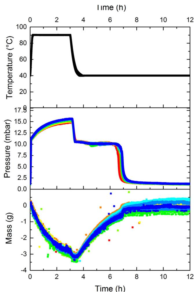
**Fig. 13.** Cyclic experiment with hydrated start material. The different colors denote different cycles. Top: temperature as function of time. Middle: Pressure as function time, slight variation in pressure. Bottom: Mass as function of time, with some variation all cycles overlap in hydration rate. (For interpretation of the references to color in this figure legend, the reader is referred to the Web version of this article.)
