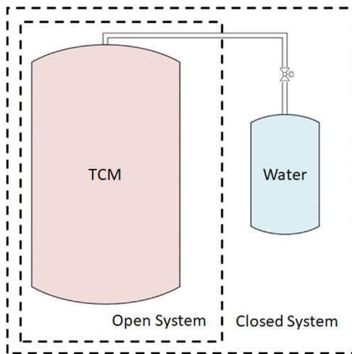
**Fig. 2.** Schematic representation of a closed and open reactor system. The closed system operates under pure water vapor conditions. In a closed system liquid water is stored inside the system and water vapor is generated internally with an evaporator. In an open system the TCM is operated at ambient pressure in the presence of inert gas (air), the water vapor is supplied to the TCM from an external source. Figure adapted from Refs. [13].
